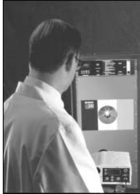
Operator calibrates a transfer standard (lower foreground) – an infrared thermometer with 0.1°C resolution – with a blackbody calibration source that provides temperatures from 600° to 3000°C.
