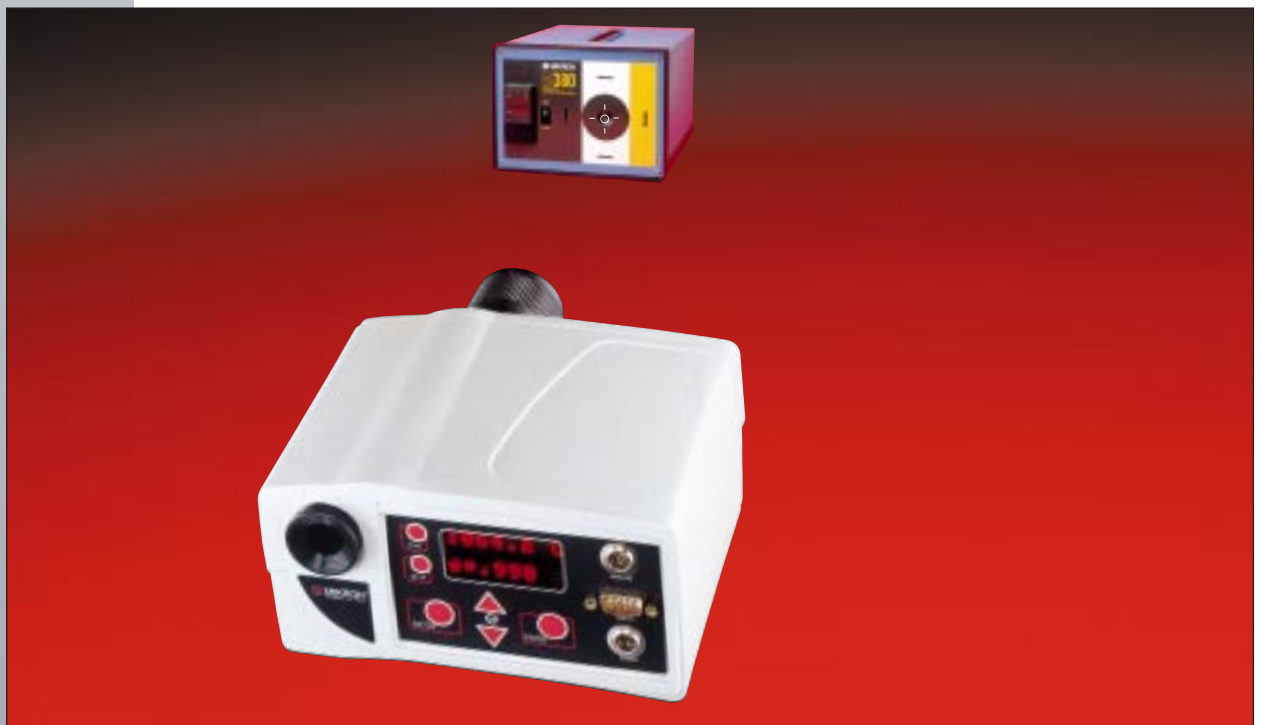
Shown above is the Model M190V-TS aimed at Model M380-AU, a primary standard Gold freezing point blackbody source.
