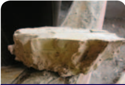
Figure 4: unscheduled forced shutdowns to clean fan. Four kiln stops in 2005
